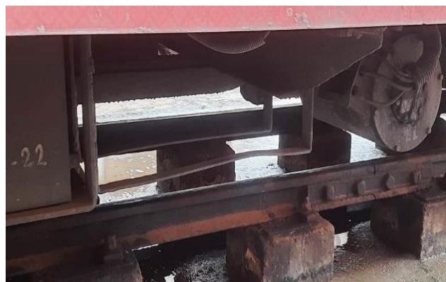
[Fig.3: Alternator Connected with ICF coach in KLK-Shimla Trains]
