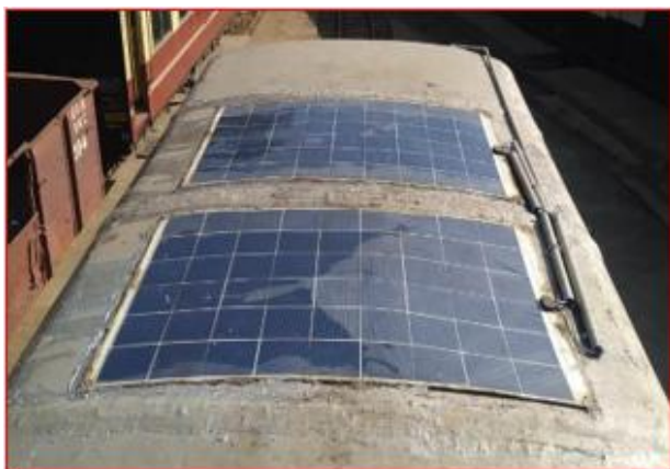
[Fig.5: Solar Panel on Roof of NG Coach/KSR]
